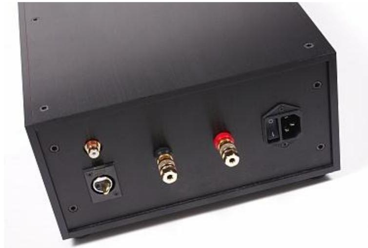
At the back side are only the essential. The binding posts are of very good quality, by Cardas.
